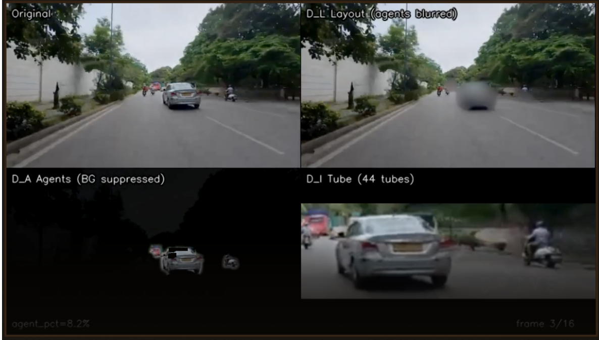
Figure 13: Automatic factor-target construction. Per clip, the pipeline derives layout D_L , agent D_A , and interaction D_I supervision by masking foreground/background and linking agent tubes.
