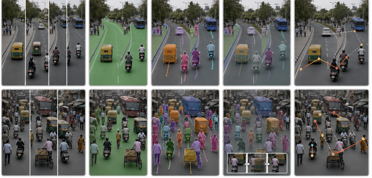
Figure 16: Conceptual end-to-end construction of FactorJEPa targets. The upper band shows the frozen teacher-side pipeline: a privacy-filtered clip is processed by DINOv2 to obtain region evidence—masks, boxes, descriptors, and confidence—which is linked into tracklets by temporal association. The deterministic structural map then produces layout, agent, visibility, and interaction targets \{T_L, T_A, T_V, T_I\} together with stop-gradient reliability weights \omega . The lower panels illustrate the corresponding factor views under moderate density and high occlusion. Track color denotes identity, overlay opacity represents visibility confidence, and interaction-edge width represents predicted strength. The scenes are synthetic and illustrate the target semantics; they are not empirical DINOv2 outputs.
