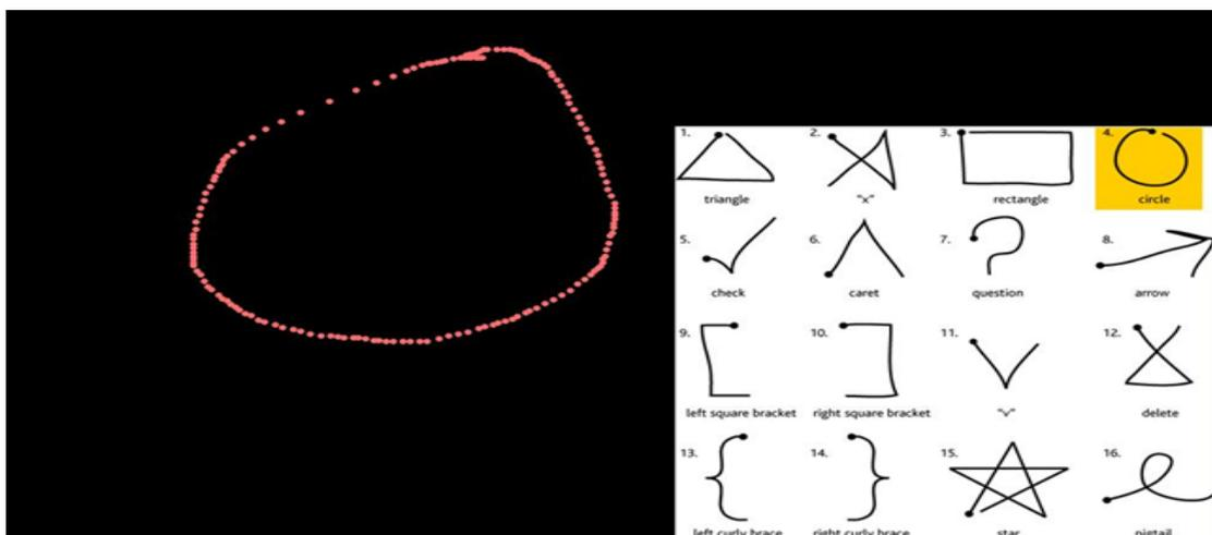
The above diagram shows templates for the gestures as registered on the screen surface. Here, a circle can be interpreted to switch on the fans. A square can be interpreted to turn off the fans. Similarly, other symbols can be used to operate on the other circuits in a home.
