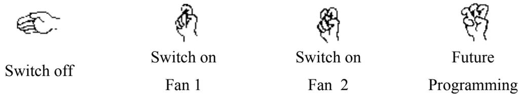
Gesture 1 is used to switch off all the fans, while Gestures 2 and 3 are used to switch on Fan1 and Fan2. Gesture 4 is reserved for future programming for complicated functions like adjusting the speed inclination (in case of a table fan) of the fan etc.
