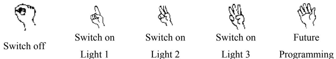
Gesture 1 is used to switch off all the lights, while Gestures 2, 3 and 4 are used to switch on Light1, Light2 and Light 3. Gesture 5 is reserved for future programming for complicated functions like dimming the light, switching it on and off in succession etc.
