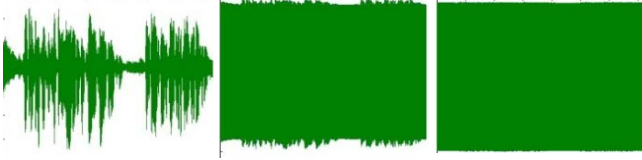
Fig 6: Original signal (Left), signal after Level 2 (Middle) and signal after Level 2 and AWGN Insertion (Right)
