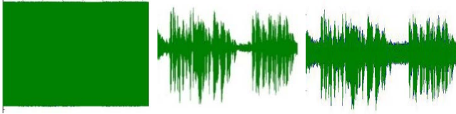
Fig 7: Received signal (Left), recovered file with high SNR (Middle) and recovered file with low SNR (Right)
