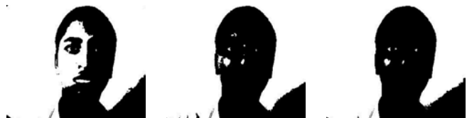
Fig. 4. B&W image of red color space (left), B&W image of green color space (middle) and B&W image of blue color space (right)
